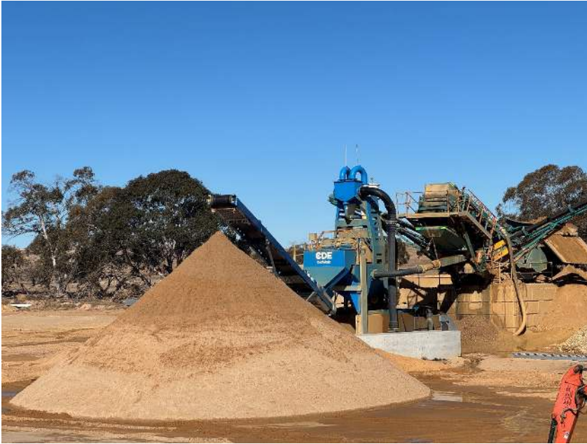
Photograph 3 , shows the current quarry operation with screening plant and sand stockpile.
